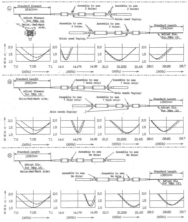
\*\* You can change Center Freq. of 7MHz by sliding the 7MHz adjust Element, without any influence to other frequencies.
